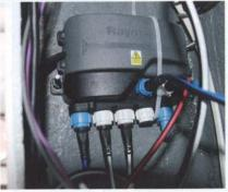
LEFT NASA wind instruments are still NMEA 0183 compatible, but you can buy a translator box to enable the data to link into NMEA 2000 system. RIGHT Raymarine's Seatalk system is effectively NMEA 2000
