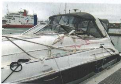
ABOVE The Doral 10m powerboat Phoenix was pushed along by the IOW ferry Red Falcon for 18 seconds
