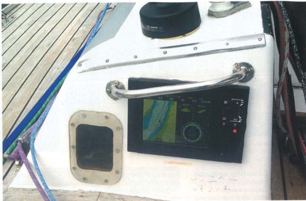
ABOVE My preference is to mount an MFD on deck and use a tablet as a repeater at the chart table below
