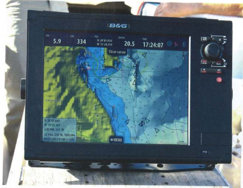
NMEA2000 displays can be used to show any data on the network – they are much more flexible than old-school electronics where each unit had a different function
