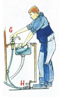
Pressurised water systems are fine, but they can't tell the difference between an open tap and a leak – so they could pump all your fresh water through a split pipe into the bilge. To conserve water on long passages it might be safer to use a hand pump (G) or, better still, a footoperated pump (H).
