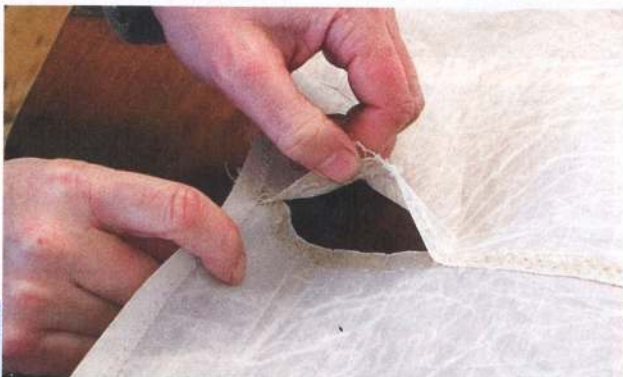
LEFT When examining sails take a careful look at the leech, which is where problems are likely to start
