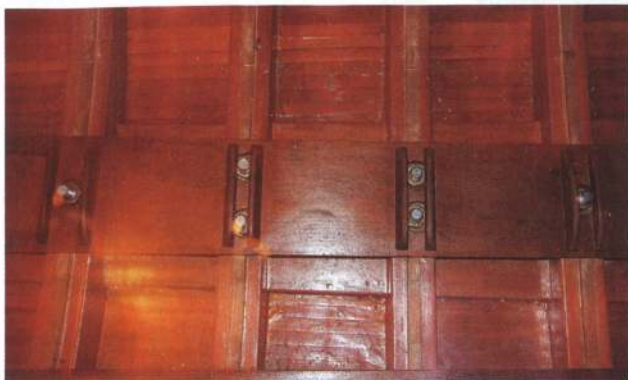
BELOW Lift the floorboards to look at the bilge. Not all will be as immaculate as this, but walk away if there's so much grot you've no chance of seeing the structure
