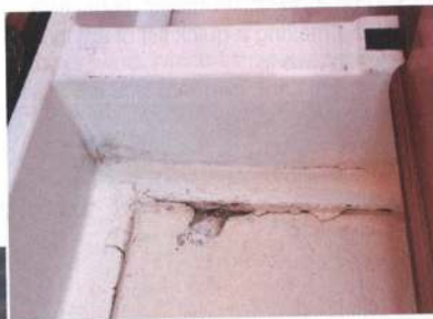
ABOVE A broken structural matrix as the result of a hard grounding
