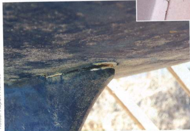
ABOVE A broken structural matrix as the result of a hard grounding
