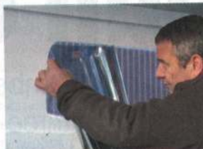
Other ways to keep a boat cool are to fit reflective film to the windows...
