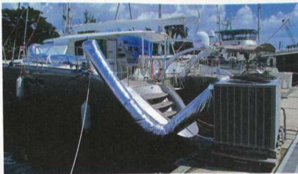
A portable aircon unit being deployed in Florida during refitting of a yacht. Without the yacht's own system in action, working below in this dark-hulled vessel would be uncomfortably hot
