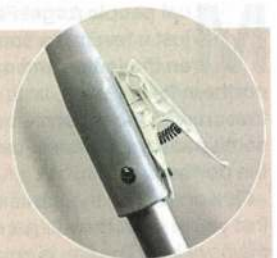
Clothes peg is glued and screwed to the boathook pole to hold a line
