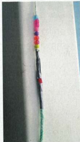
Differing sizes of plastic bracelet beads helped this halyard over a mast sheave
