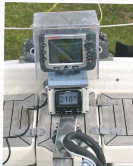
A coaming shelf supported by a waterproof box makes a perfect position for helm instruments
