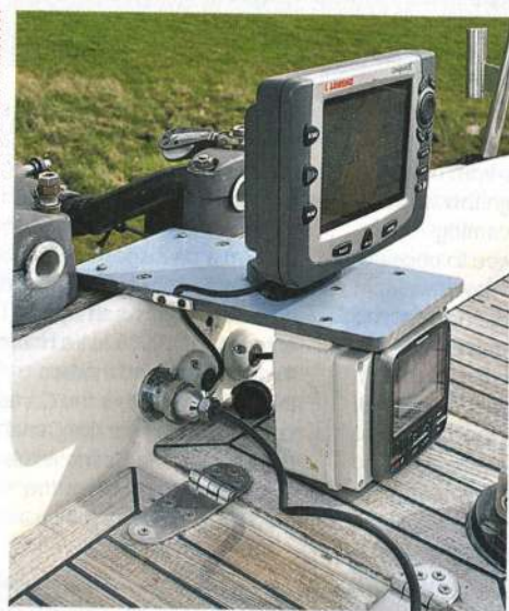
A coaming shelf supported by a waterproof box makes a perfect position for helm instruments
