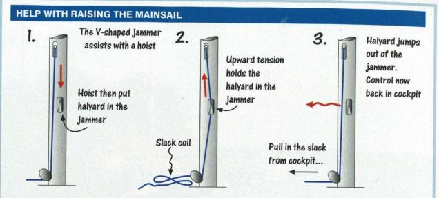
An 8oz Dacron mainsail on a 38ft cruising boat is a heavy piece of gear. If the halyard passes round a turning block at the foot of the mast, then through an organiser on the coachroof then through a closed clutch, just forward of the winch, there is enough extra friction load by the time it reaches the winch to make raising the sail quite a
