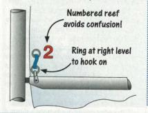
makes hooking on really easy. This is crucial when you are taking a reef on your own. Once I have the slack on the reefing line pulled in, I tighten the halyard until the two red marks are just at the winch, which gives me the right halyard
