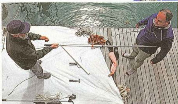
A sprung sling deployed attached to a boathook. Pulling on the pole side string decreases the size of the loop
