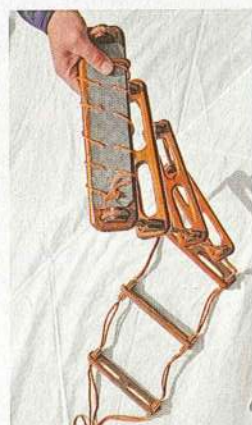
The bottom step of Noel's ladder is weighted, and hangs 5ft below sea level when tied to the toerail
