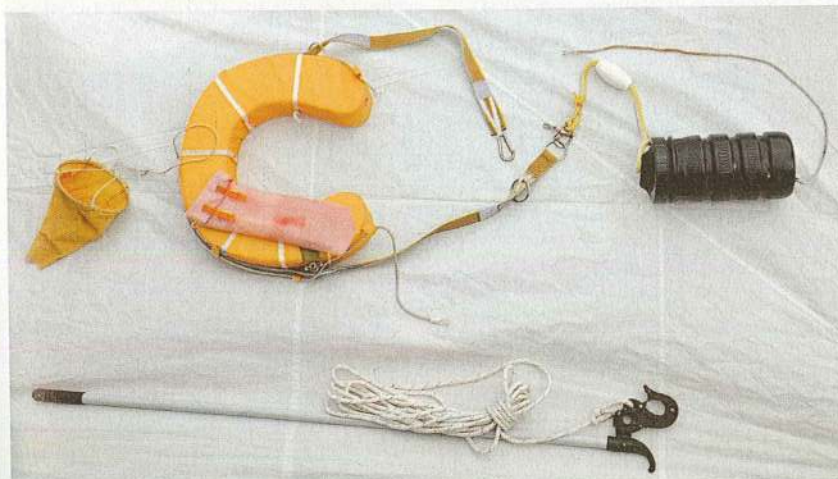
Note the open drogue, a sling round the horseshoe with an easy-release clip if being towed and a 30m line with reflective tape for visibility at night in a canister
