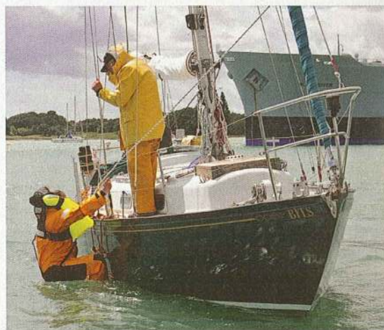
Kieran was able to board but it's safest to use the ladder with the hoist or a halyard as a safety line, to take some of the sodden weight of the MOB
