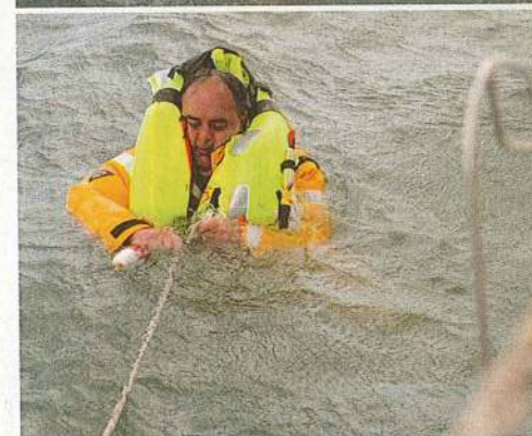
Despite his inflated lifejacket, Kieran easily passed the sling around his back and could see the clip to refasten it
