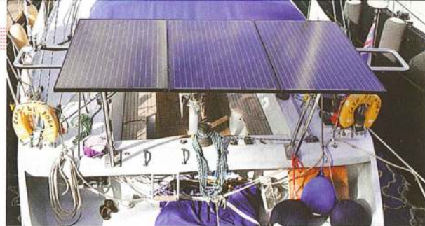
CLOCKWISE FROM TOP Three different methods of topping up your batteries without using your engine: solar panels, a hydro generator and a wind generator
