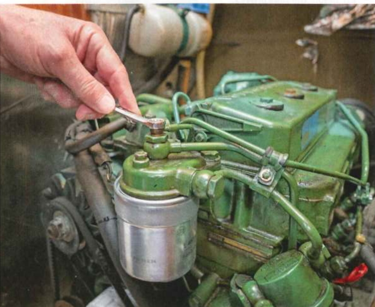
Where is the secondary fuel filter on your engine, and which spanner of the dozen you have in your tool kit is the right one to bleed it?
