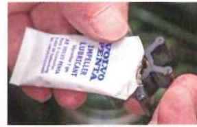
The new impeller and its washer will need lubrication, and in this case it's been supplied
