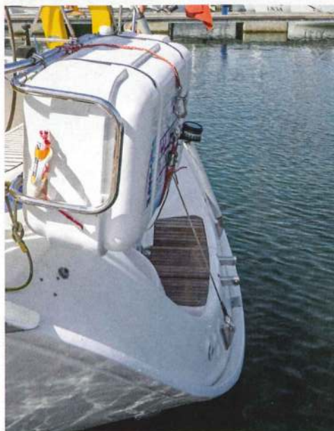
The perfect mounting for a liferaft: no heavy lifting and always accessible – even if inverted
