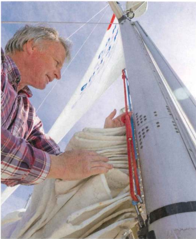
Is your mast track gate high enough to allow the trysail to be bent on? How long a tack stop do you need to keep the sail flat?
