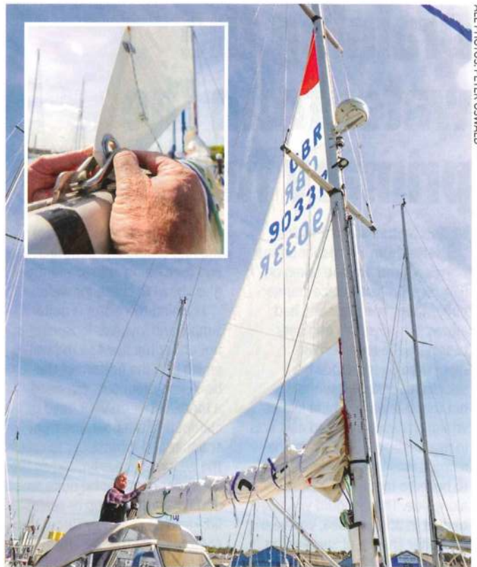
I prefer the clew on the boom as I can use the outhaul to flatten the sail, work to windward, and depower with the mainsheet if needed
