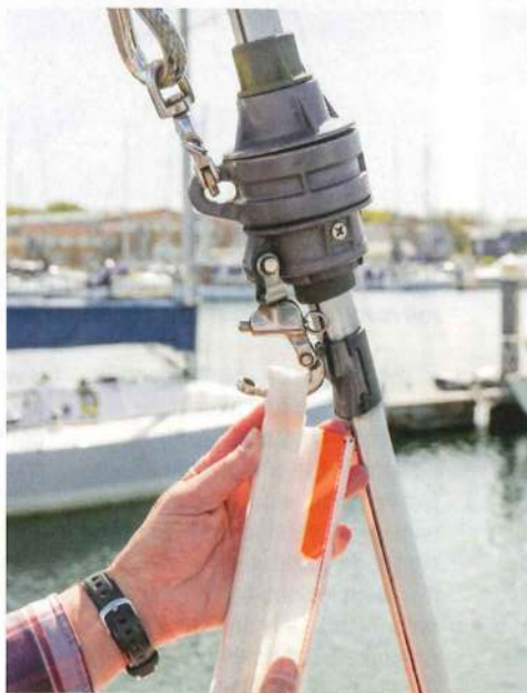
With a single forestay I need to unbend the genoa to slide my storm jib's bolt rope into the headfoils
