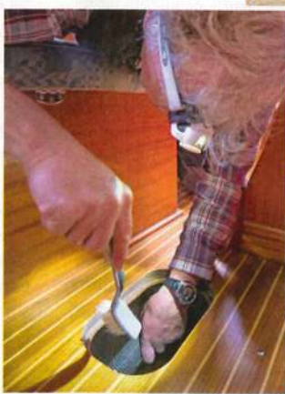
How long would it take you to locate your strumbox, and find the right tool to clean it, with the sole boards awash?
