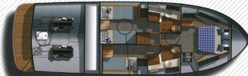
The location of the generator away from the cabins keeps noise levels to a minimum
