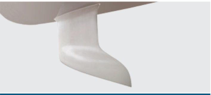
Shallow draft L-shape keel (1.37 m), cast iron
