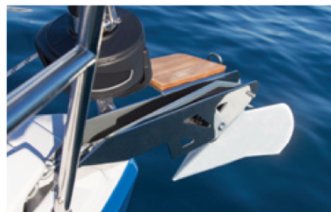
Anchor arm with roller and teak step, Anchor, Delta 10 kg, with 30 m galvanized chain, 8 mm
