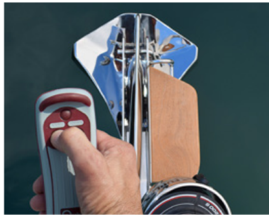
Anchor windlass, electrical with remote control
